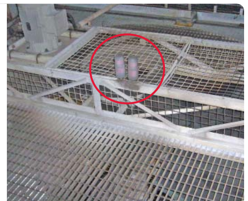
Lubrication system: 2 x perma STAR VARIO 120 cm 3
